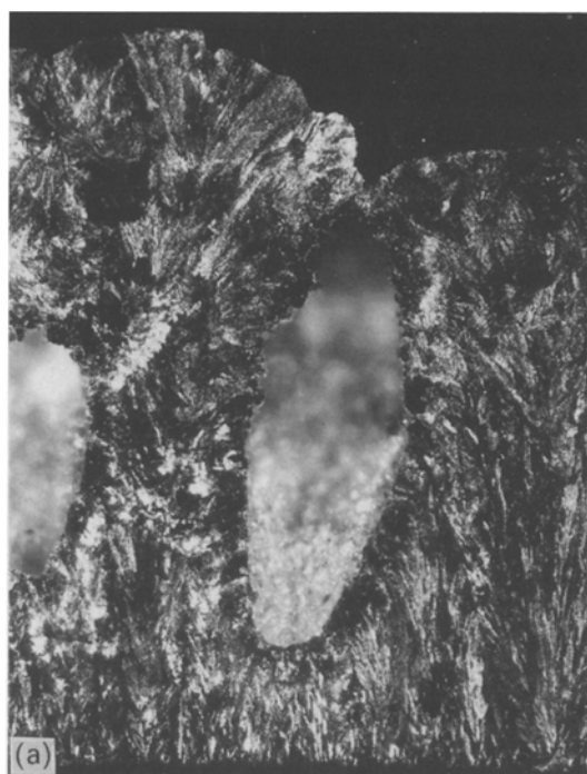
Fig. 1. Photomicrographs of a cross-section of cathodic zinc deposits, polarized light (63 \times ): (a) without surfactants; (b) D1 + D2; (c) D1 + D2 + D3.
